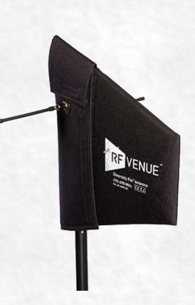
The patented Diversity Fin® is a multi-purpose antenna for wireless microphones that reduces dropouts using a cross-polarized design. It combines one LPDA and one dipole antenna in an orthogonal...
